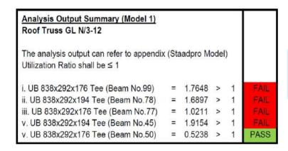
In overall, the analysis is FAIL. Therefore, solar panel are not recommended to install on the top of the roof.
