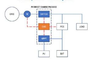
In December 2024, LEM successfully deployed a DC-Coupled Solar Photovoltaic (PV) and Battery Energy Storage System (BESS) in Pampanga, Philippines. By utilizing a DC-coupled configuration, the system achieves **higher efficiency** compared to conventional AC-coupled setups, as energy flows directly from the PV to the BESS with reduced conversion losses. This ensures customers gain maximum value from their renewable energy investment while supporting a sustainable and reliable power supply.
