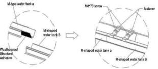
A tailored solution was provided as the client faced severe rooftop leakage that would normally require costly repair or replacement. An innovative M-Type Water Tank System was integrated to redirect rainwater to gutters, resolving the issue without roof replacement. The system now delivers up to **72% consumption offset** in monthly TNB bill and has outperformed expectations, **generating 108% above designed output**.
